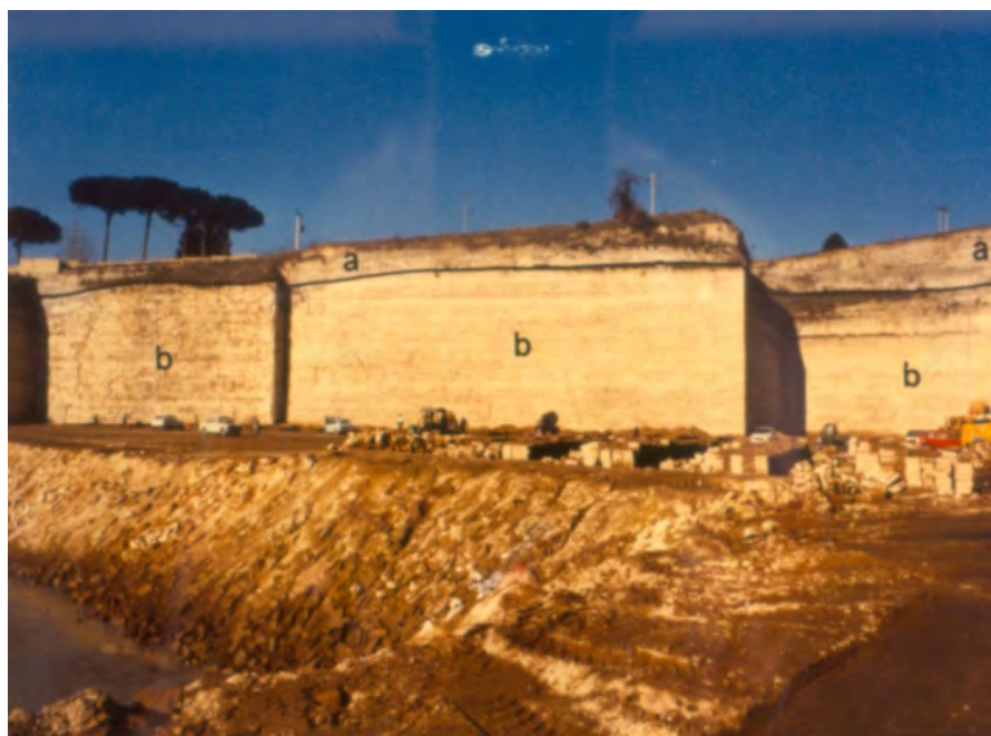
Figure 4 – NYT quarry in Quarto (see Fig. 3). a : pozzolan (unlithified original volcanoclastic material); b : Neapolitan yellow tuff.
