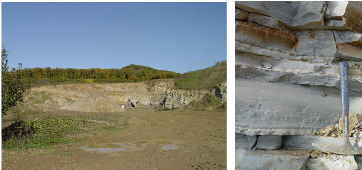
Poljanska quarry: (left) general view; (right) typical laminated carbonate-analcime sedimentary rock.
